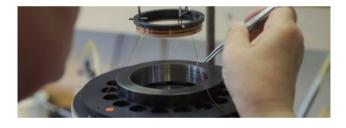
The disc does not move pistonic, like a normal driver, but the vibrations travel through the material as transversal waves, so called 'bending waves'. The thickness of the disc increases towards the
