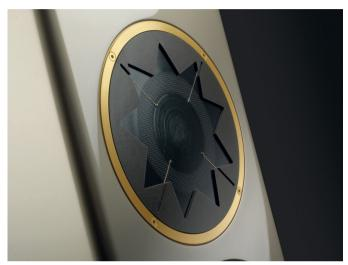
Although the Manger Sound Transducer is able to reproduce down to 80 Hz, the crossover in the p2 has been configured to filter all frequencies below 340 Hz from the Manger driver. Most low frequencies are thus handled by the woofer. This avoids forcing the Manger driver to behave pistonic and allows for a more accurate and simpler crossover. The complete midrange and high frequencies are handled by the Manger Sound Transducer without any additional filters.
